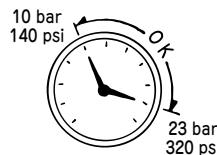
**OPERATE WITHIN THE PROPER AIR PRESSURE RANGE**
